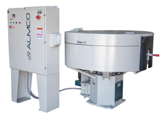
Gate Clearing Feature for Internal Separator: The gate clearing feature reduces the chances of parts getting caught between the media gate and the screen frame. This option momentarily reverses the tub while raising the media gate to clear the area under the screen.
