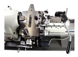
Six Station Turret: The turret tool holder diameter16mm slide travel 9mm.
