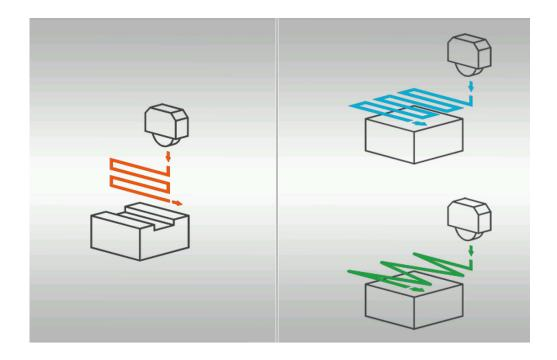
Plunge Grinding, Surface Grinding & Crisscross Grinding available on the Perfect DT Series Surface Grinding Machines.
